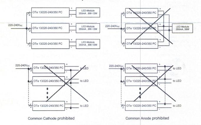
The installation of two or more OPTOTRONIC® OTe 13/220-240/350 PC Power Supplies with common "-" or "+" wiring by the intention to save wire to LED modules is prohibited, in order to avoid exceeding the maximum allowed system touch current levels on the accessible parts of the installation.
